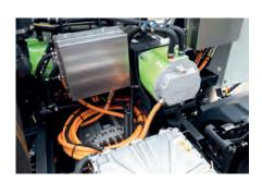
**INVERTER AND ELECTRIC PTOs**Liquid cooled, high voltage three phase inverter controlled electric drive motors for jetting and vacuum pumps.
